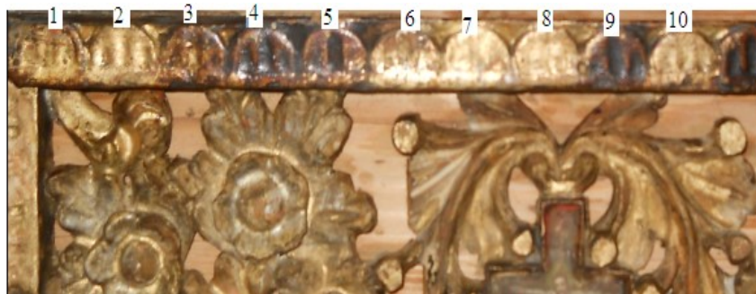
Fig. 4. Cleaning tests for the gold leaf covered carved wood, with simple and mixed solutions (E1, E10)
