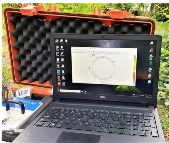
Figure 1. Arbotom ABTO 5S, 2D/3D-Sonic-Tree-Tomography (Foto: Enescu R.)
