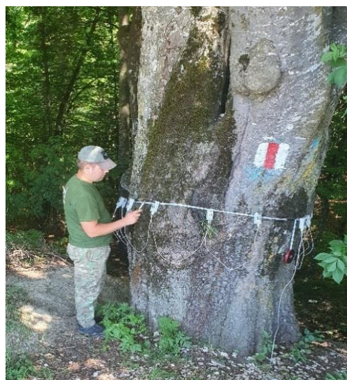
Figure 2. The sensors attached to the trunk by the pins (Foto: Enescu R.)
