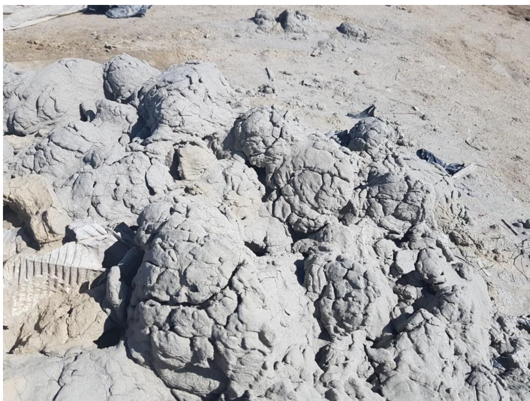
Figure 1. The crumbling aspect of Miocene Marl in Fez vicinity (Morocco)
