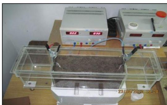
Fig. 1 - Experimental installation of electro-flushing (top view)
